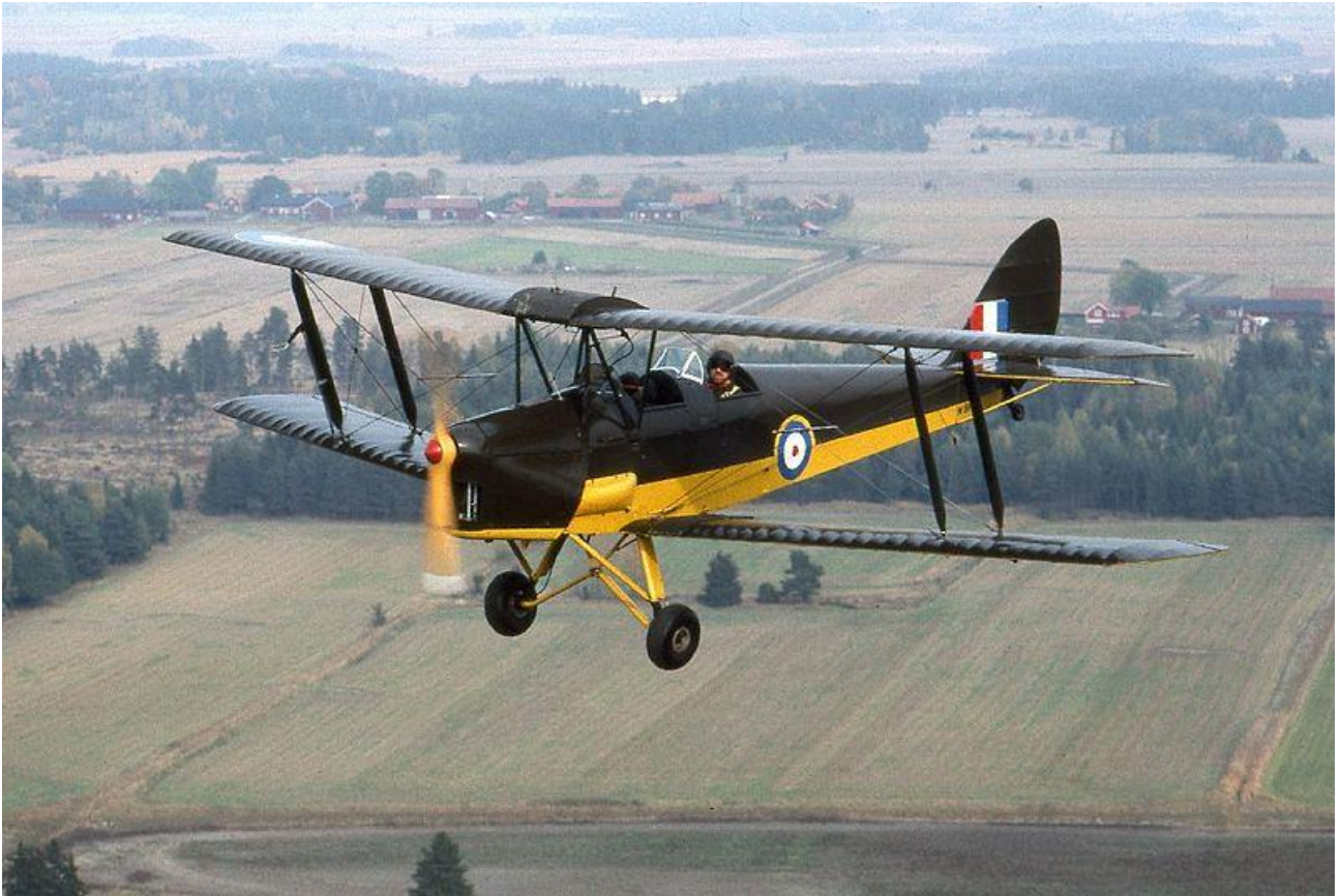
de Havilland DH.82A Tiger Moth (Tiger Moth II) Fitted with the Gipsy Major 130 H.P.
